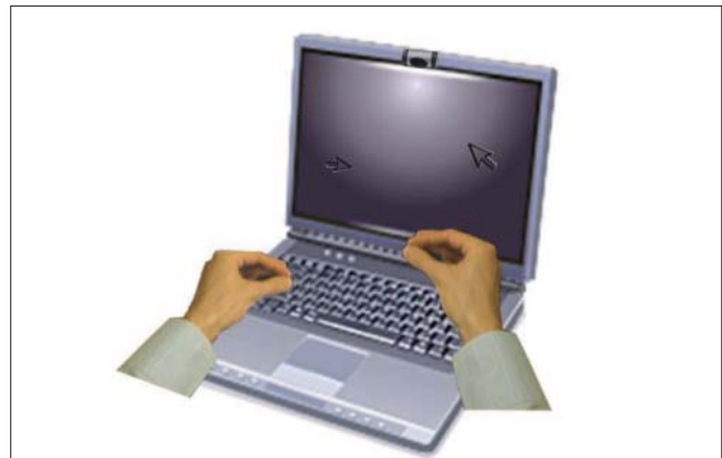
Figure 12: System setup. A camera is mounted on top of the monitor and is directed at the user's hands. A pointing device can be implemented by foreground segmentation and shape analysis.
